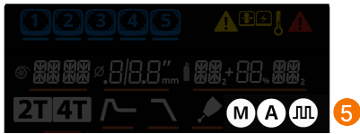
5. MIG welding process indicators
